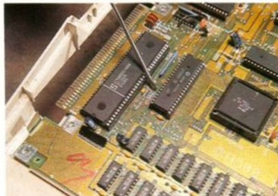
On revision 5 boards, JP2 is further away from the front of the board, but it's still fairly accessible.
